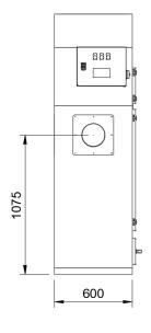
Front and side view B 1000 PF - Cartridge filter unit
